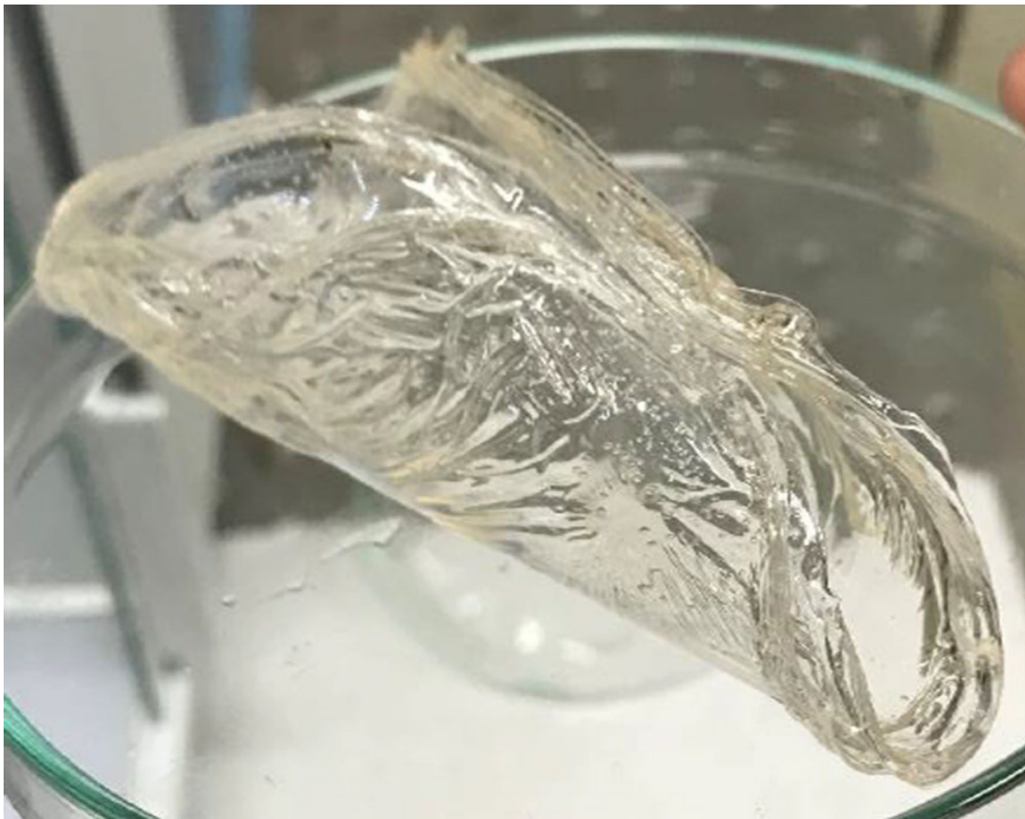
Figure 4 - Semi-irreversible contracture of thick PVA hydrogel
